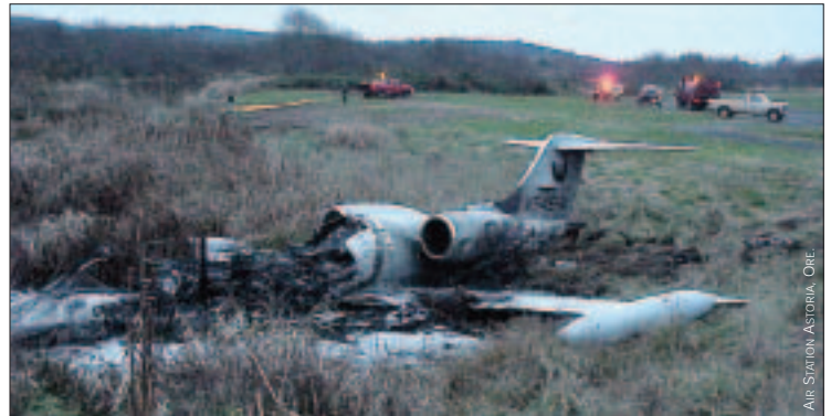
The remains of a downed Lear 36 jet after colliding with an elk.
